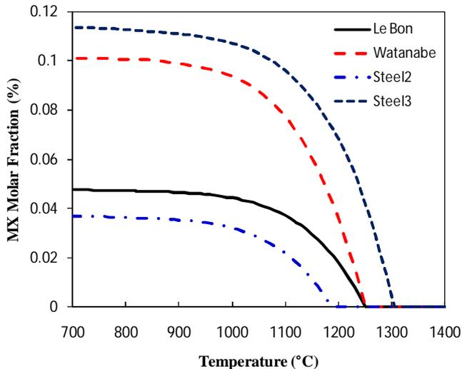
Fig. 3. Molar fraction of MX in the four steels calculated using JMatPro.
