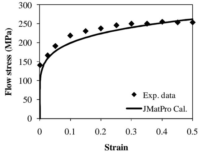
Fig. 2. Flow stress curve at  $950^\circ\text{C}$  at strain rate  $10 \text{ s}^{-1}$ , experimental data from Ref. 24.
