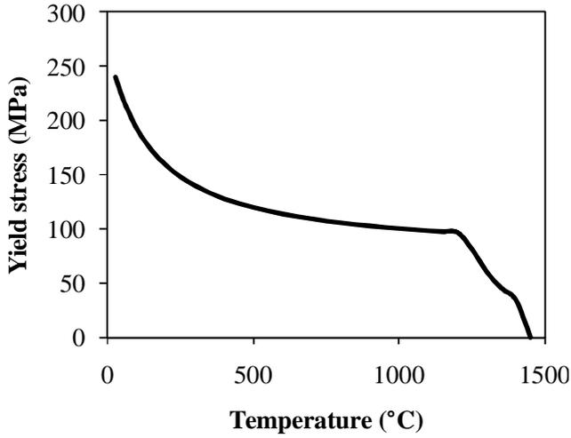
Fig. 1. Yield stress of austenite as a function of temperature calculated at strain rate  $10 \text{ s}^{-1}$ .
