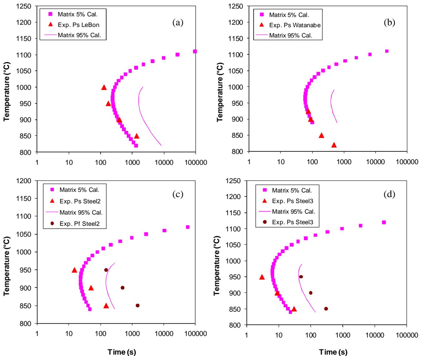
Fig. 5. Calculated TTP curves for four microalloyed steels in comparison with the experimental data from: (a) Le Bon,<sup>1</sup> (b) Watanabe,<sup>2</sup> (c), Steel2 of Hansen et al.,<sup>5</sup> and (d) Steel3 of Hansen et al.<sup>5</sup>
