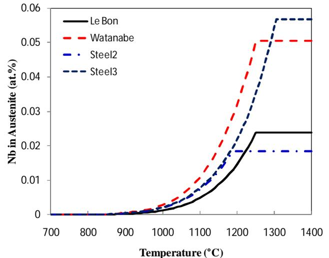
Fig. 4. Nb in austenite in the four steels calculated using JMatPro.
